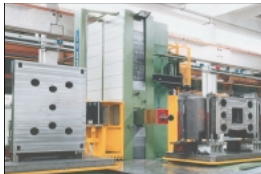
Boring and milling machine model FRAL 515 complete with two rotary traverse tables typ TRT 150, automatic tool changer 90 places and traverse moveable pick up outside machine's working area.
