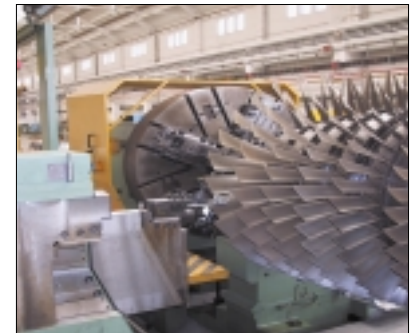
Leonard 80 CNC lathe, for trimming operations on assembled turbine rotors. Swing up to 4,000mm, weight up to 200 tons.
