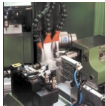
A grinding operation controlled by Marposs UNIMAR in process gauge, Marposs Wheel Balancer, ultrasonic gap eliminator and MIDA™ touch probe for flagging.
