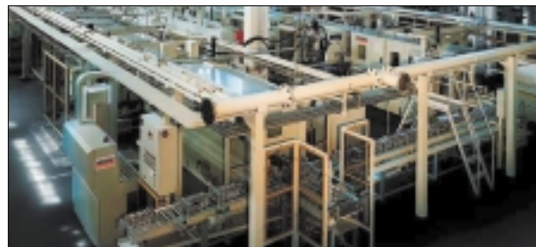
Cylinder head cubing lines.
