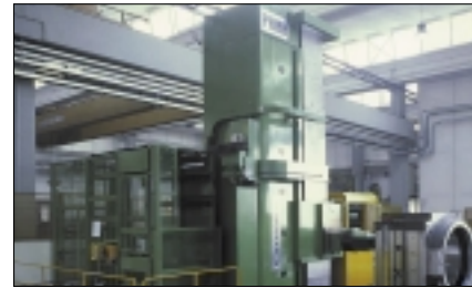
Speedram 2 with universal milling head, rack magazine 140 pockets and rotary table 45 tons.
