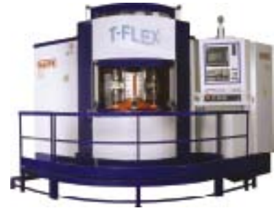
T-FLEX42 NC flexible two-spindle transfer machine for the production of complex parts of every shape in small/medium batches requiring machining from 4 or more positions
