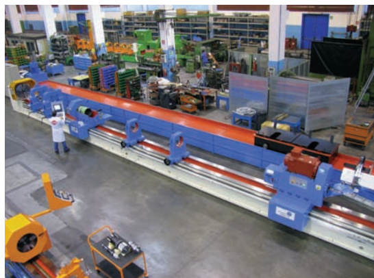
Deep Hole Boring Machine GGB 560 CNC 520x7000 with Bottle Boring System
