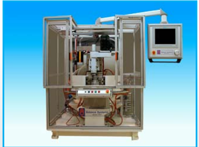
BVK30 - DISK SHAPED PARTS BALANCING MACHINE
