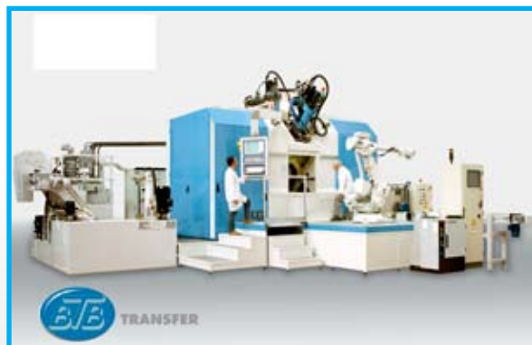
Multicolor flexible transfer machine with 19 machining centers including an integrated tool change
