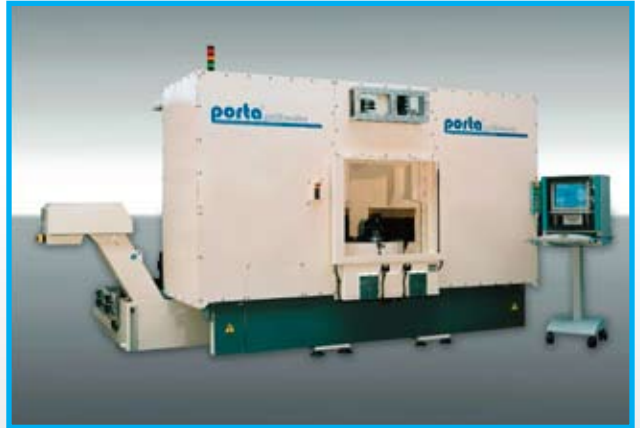
Multicenter M-04-03 4 Pallets – 3 Working Centers – 75 Tools
