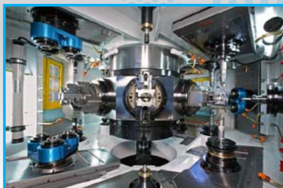
Flexible machine with CNC rotating chucks in 360,000 positions. Equipped with 3-tool 4-Axis Multi-Process. Modules (patented). Tool change time in less than 0.4 seconds.
