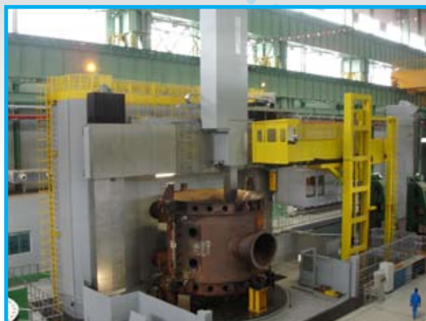
Vertical lathe model AP 120 TM 8000: big machining for energy sectors: turbines and nuclear components.
